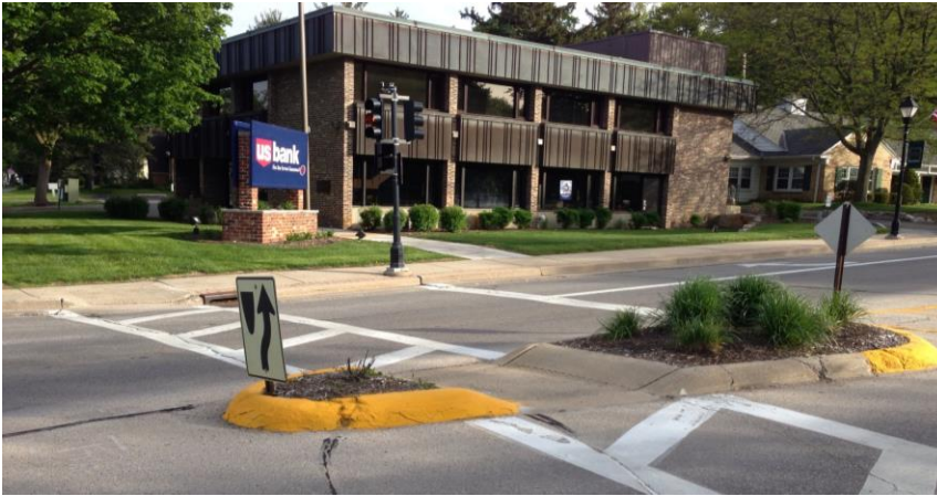
Figure 4: Typical Pedestrian Median Refuge Island
