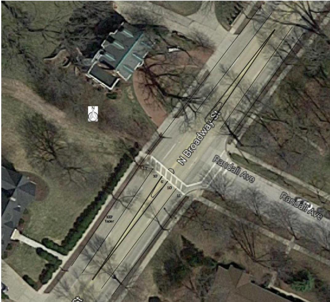
Figure 18: Pedestrian Median Refuge Island Design
