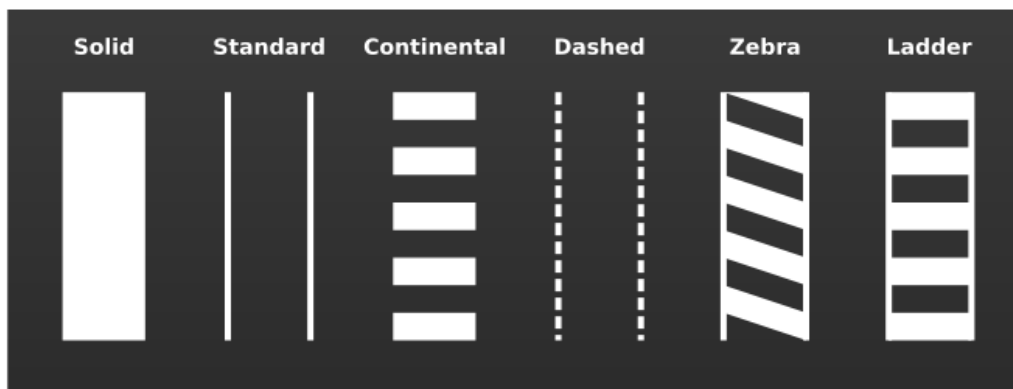
Figure 2: Crosswalk Striping Patterns
