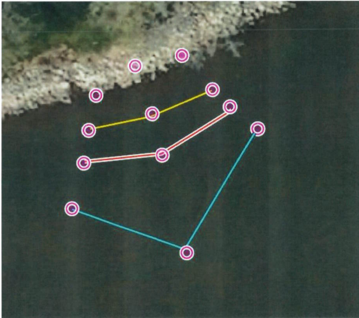
This figure shows the 2.5 ft – 3.5 ft contours at 6 inch increments along the three transects that were measured on the south point and used to design the south reef.
