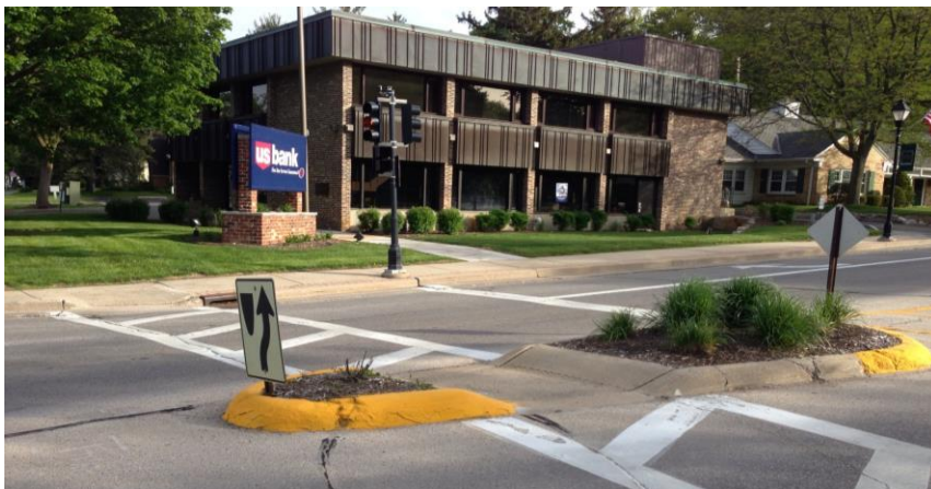
Figure 4: Typical Pedestrian Median Refuge Island
