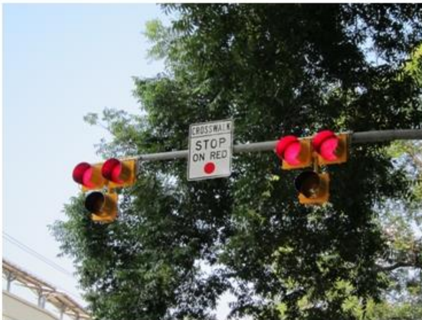
Figure 11: Pedestrian Crossing Hybrid HAWK Beacon
