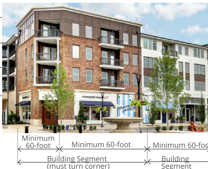
Figure 9-1. Major and Minor Materials on a Facade
