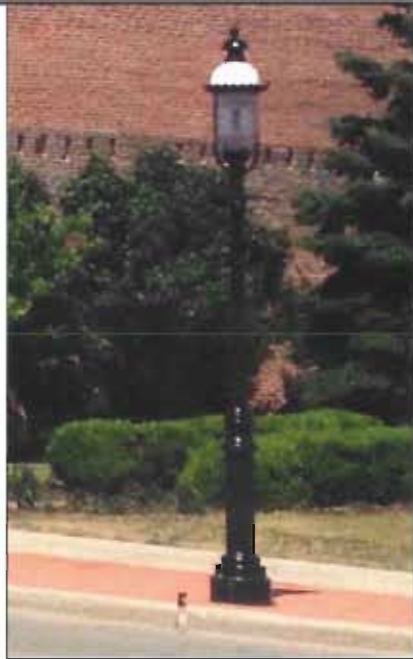
TYPICAL PARKING LIGHT POLE: 7 NEW NEW LIGHT POLE FIXTURES TO BE INSTALLED, FIXTURES TO MATCH EXISTING CITY STREET LIGHTS, TYP.
