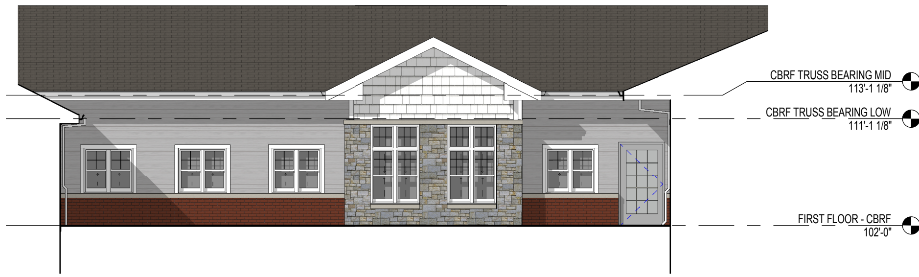
S2 A401 COURTYARD ELEVATION - SOUTH 2 1/8" = 1'-0"
