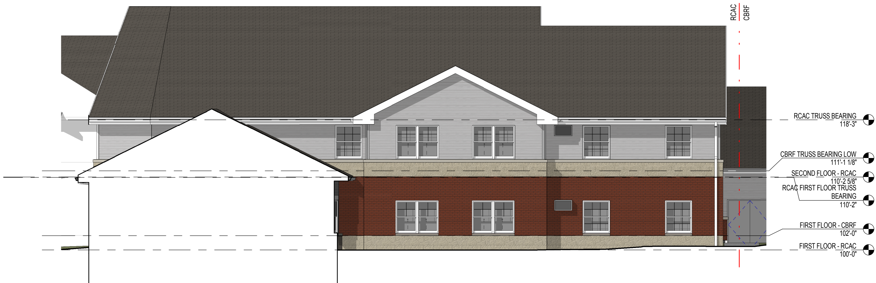
A2 A400 NORTH ELEVATION - RCAC ADDITON 1/8" = 1'-0"
