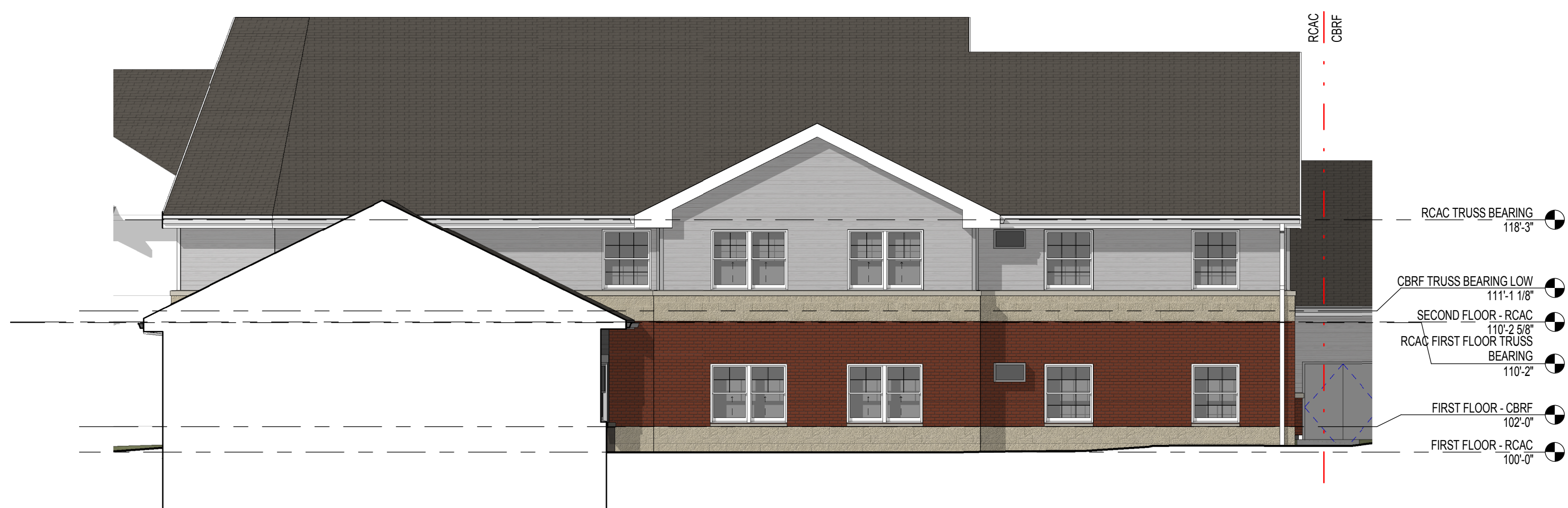
A2 A400 NORTH ELEVATION - RCAC ADDITON 1/8" = 1'-0"
