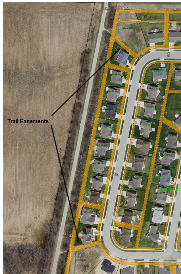
Figure 3-1. Existing trail access easements.
