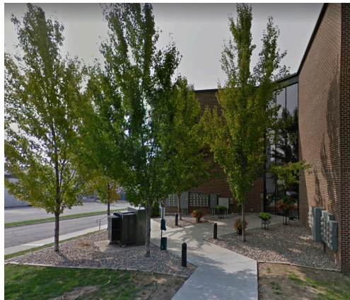
Figure 3-34. Examples of Poorly Located Utility Appurtenances without Screening on Primary Streets: NOT PERMITTED
