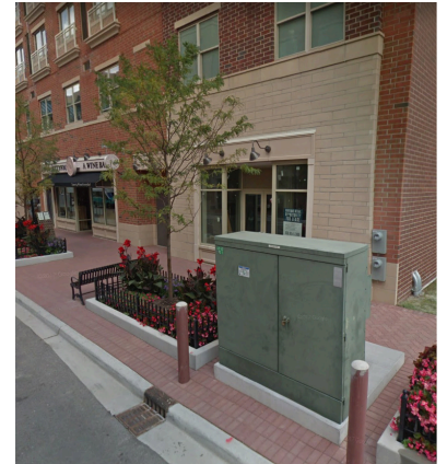
Figure 3-34. Examples of Poorly Located Utility Appurtenances without Screening on Primary Streets: NOT PERMITTED
