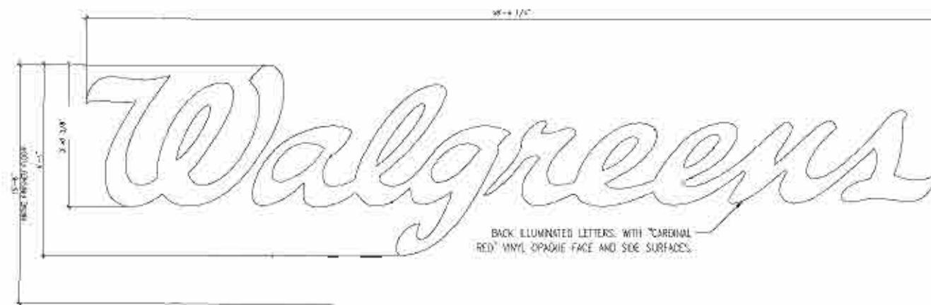
4 LED BACKLIT WALL MOUNTED SCRIPT SIGN 3/4" = 1'-0"
