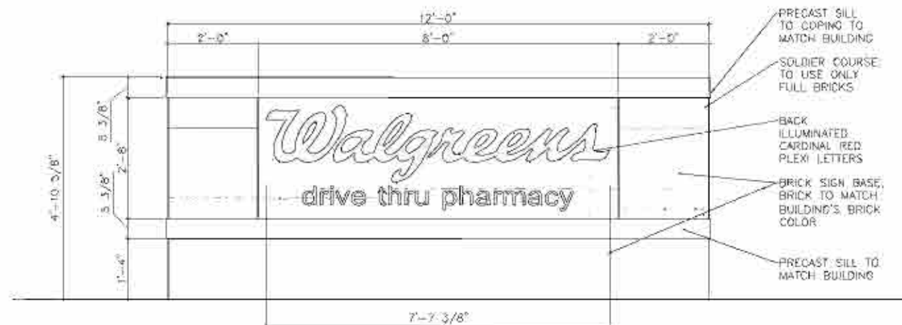
10 LED BACKLIT MONUMENT SIGN ELEVATION 1/2" = 1'-0"
